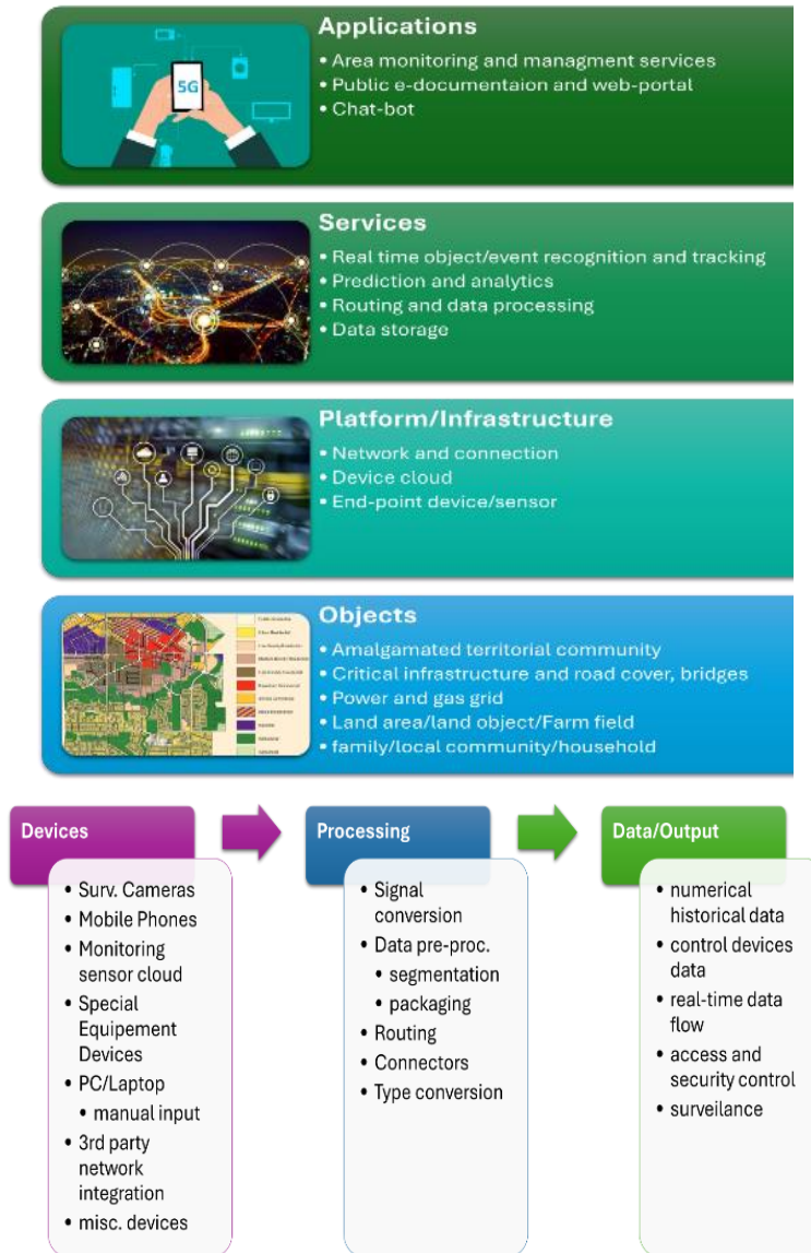
Fig. 3. IoT Area Management System Model – components and data
